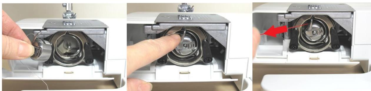
**B (horizontal bobbin case):** put the bobbin correctly in the machine.
