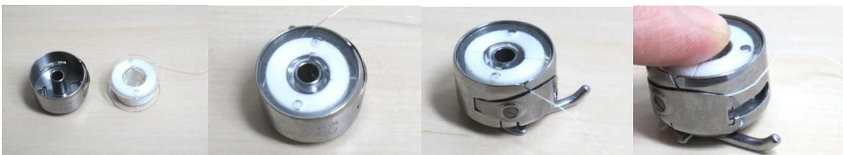
You can test the tension by hanging bobbin and bobbin case, keeping the thread between your fingers. Move your hand up and down slowly the bobbin and bobbin case should drop about 1 cm.
