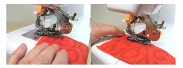
Slide the fabric to which you want to attach the ruffled band between the foot.
