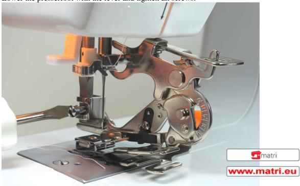
Before starting to sew, check the foot if all screws are tightened and the foot is in the right position so the needle fits in the hole and doesn't touch the foot. Turn the handwheel to check! If the needle doesn't fit in the hole of the foot, loosen the screw and push the foot a little bit to the left or right.
