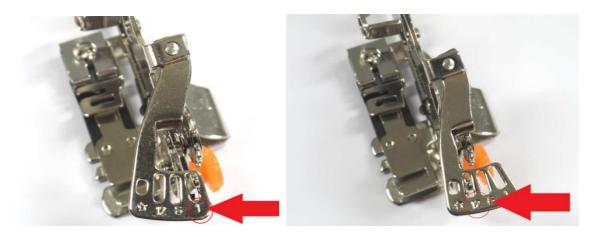
You can also adjust the depth of the ruffles (between 0 and 8, 0 having almost no depth, to 8 having the most depth. To adjust, turn the orange button, tighten the screw afterwards.
