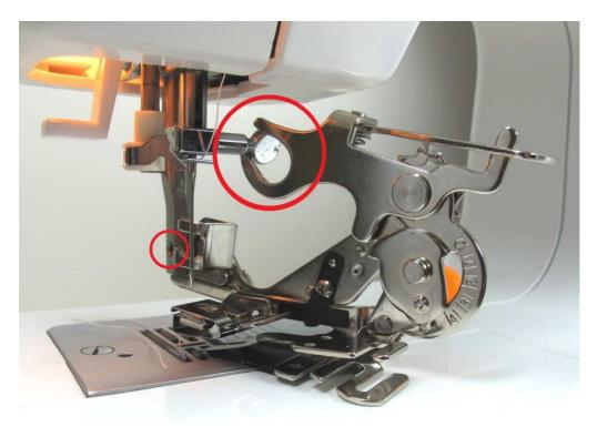
Lower the presserfoot with the lever and tighten all screws.
