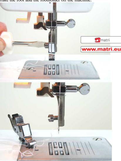
Attach the ruffler foot, be careful to fit the forked part around the screw of needleclamp. On the left side, the foot has to fit around the presserfoot bar so the screw on the foot can be secured.
