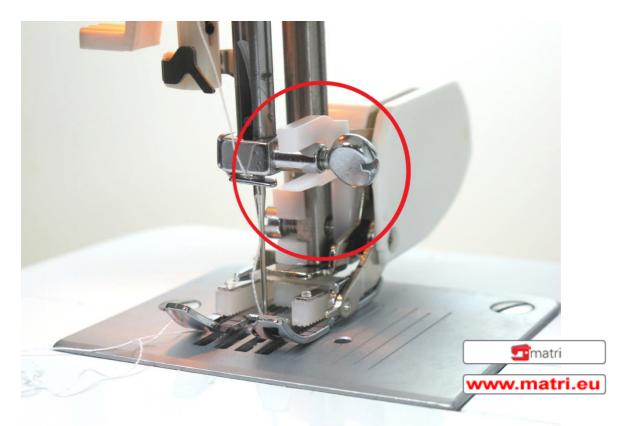
On the left side, the food needs to fit around the presser foot rod so the screw can be tightened correctly.
