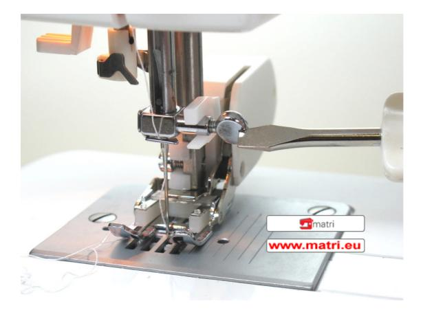
Before starting to sew check that everything is tightened correctly. Turn the handwheel and check that the needle doesn't hit the foot.
