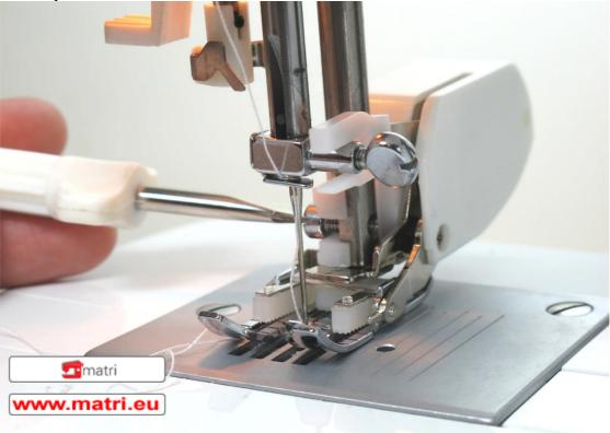
Lower the foot with the lever and tighten all screws.
