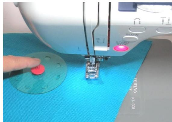
Choose a stitch. Because the fabric is fastened on the pin, the fabric will turn. Don't use a piece of fabric too big, If the fabric touches the machine, it will not turn smoothly.
