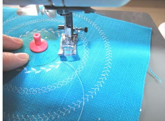
You can also repin the fabric, so you can make circles with different centerpoints. Or try making parts of circles.
