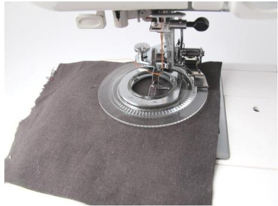
Start sewing. After a few stitches, pull the threads to the top and cut them short, so the threads don't get tangled while turning the fabric. The fabric will turn because of the foot.
