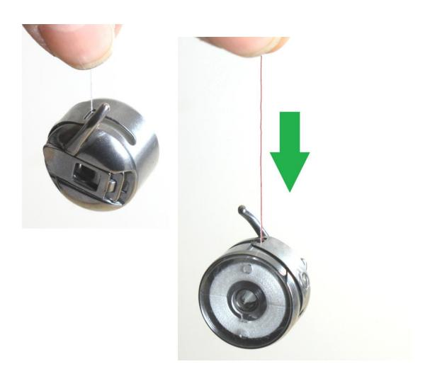
If the tension is ok, you can put bobbin and bobbin case in the machine with the « finger » up. Open the little cover on the bobbincase to be able to put the bobbincase in the machine. Close the cover. Pull the thread, the bobbin case should stay in the machine and not turn.
