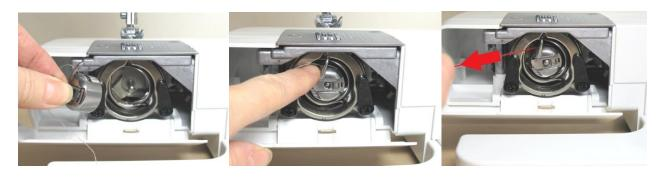
**B** (horizontal bobbin case): put the bobbin correctly in the machine.
