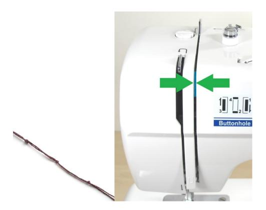
Rethread the machine again. Pull the thread to test the tension. If all is well, thread the needle.
