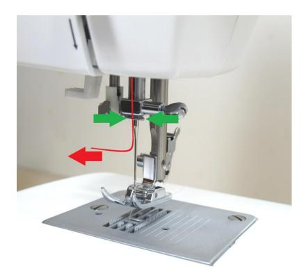
Just after having put the thread behind the hook, just before threading the needle, lower the pressure foot.
