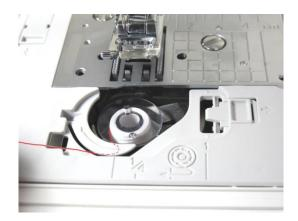
Pull the thread through the groove while keeping the bobbin in place. The bobbin thread follows a path with a tension system. If you pull the thread, the bobbin should stay in place, even if the cover has not been put in place. The bobbin turns. Rethread if the bobbin is not staying in place.
