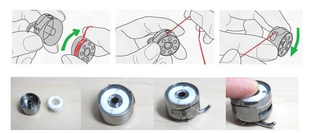
You can test the tension by hanging bobbin and bobbin case, keeping the thread between your fingers. Move your hand up and down slowly the bobbin and bobbin case should drop about 1 cm.
